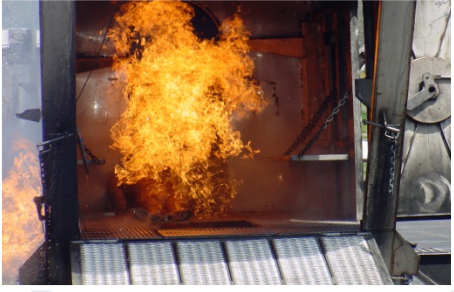
Fireball of propane fed flames coming out the ramp at the rear of the plane.
